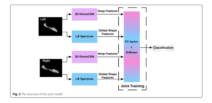
Figure 3 illustrates the architecture of direct combination of CNN features and shape features.
